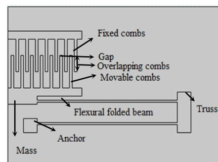
Fig 1. Structure of interdigitated comb drive MEMS resonator
