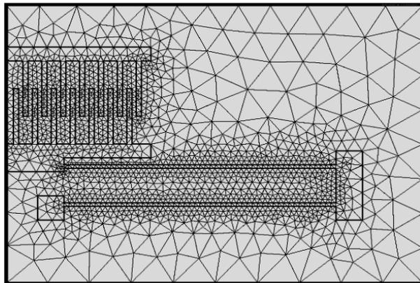
Fig 2. Free Triangular Mesh (coarse)
