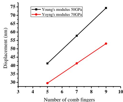
Fig. Number of combs vs displacement
