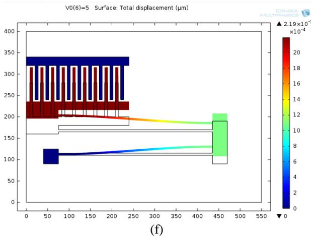
Fig 3. Illustration of electric potential and total displacement
